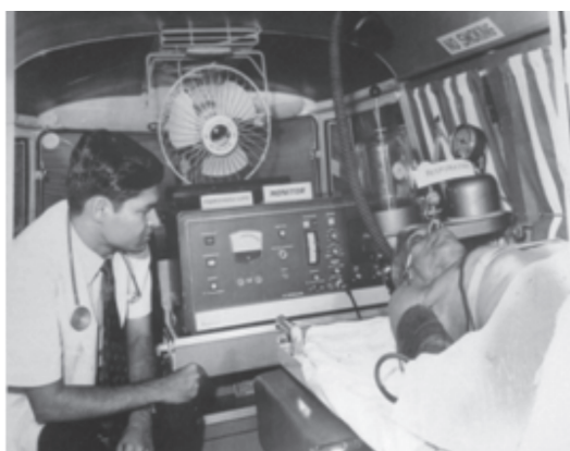
Fig. 3 : Interior of the mobile coronary care unit with cardioscope and other instruments
