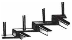
Non Slip Tread Cap in Stairs
